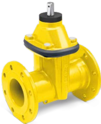
Alternative for gas DN 40–300, PN 10–16 as per EN 13774
